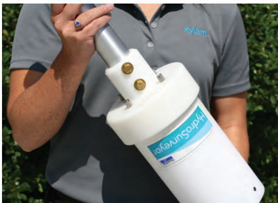
Custom designed Delrin/aluminum fixture to facilitate mounting the HydroSurveyor over the side of a boat.
